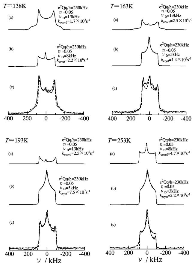
**Figure 6.** Observed and theoretical  $^2\text{H}$  NMR spectra for  $\text{Sm}(\text{NO}_3)_3 \cdot 6\text{D}_2\text{O}$ . (a) The theoretical spectra for the coordinated water molecule. (b) The theoretical spectra for the crystallization water molecule. (c) The solid lines show the observed spectra. The broken lines show the theoretical spectra obtained by the combination of (a) and (b) in the ratio 2:1.
