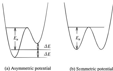
**Figure 3.** Potentials for the 180° flip of the water molecule in  $\text{Sm}(\text{NO}_3)_3 \cdot 6\text{D}_2\text{O}$ . (a) and (b) show the asymmetric and symmetric double minimum potential, respectively.
