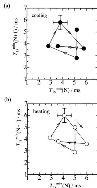
**Figure 8.** Return maps for the minimum values of  $^2\text{H}$  NMR  $T_{1s}$  for annealed  $\text{Sm}(\text{NO}_3)_3 \cdot 6\text{D}_2\text{O}$ . The minimum values of  $T_{1s}$  at the  $(N+1)$ th run are plotted as the ordinate and at the  $N$ th run as the abscissa. (a) and (b) show the results of the cooling and heating processes, respectively.
