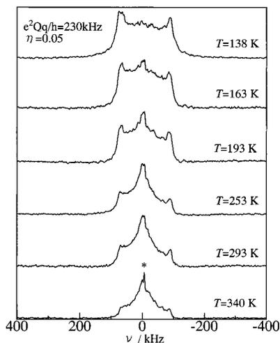
**Figure 1.** Observed  $^2\text{H}$  NMR spectra for  $\text{Sm}(\text{NO}_3)_3 \cdot 6\text{D}_2\text{O}$  using the shift-compensated pulse sequence. The asterisk shows the sharp component of the spectrum arises from free  $\text{D}_2\text{O}$ .
