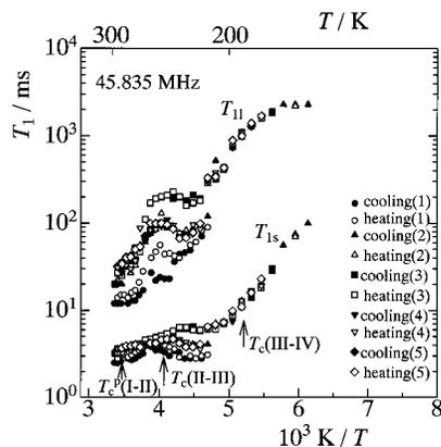
**Figure 7.** Temperature dependence of  $^2\text{H}$  NMR  $T_1$  for annealed  $\text{Sm}(\text{NO}_3)_3 \cdot 6\text{D}_2\text{O}$  in several measuring runs of cooling and heating.  $T_c(\text{II}-\text{III})$  and  $T_c(\text{III}-\text{IV})$  show the transition temperature determined by the present DTA measurement.  $T_c^p(\text{I}-\text{II})$  shows the phase I-II transition point for the protonated compound.
